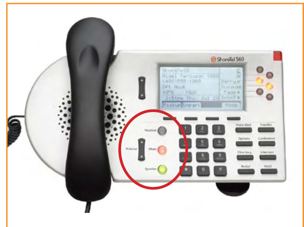
Figure 4: It’s easy to switch between a handset, headset and speaker. Plus, bright indicator lights make it easy to see if a person is on the phone.
