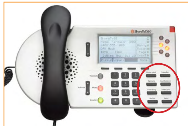
Figure 12: ShoreTel has grouped together the feature keys for the most common features for consistent, easy access. This includes transfer, conference, intercom, hold, voicemail, options, directory and redial.
